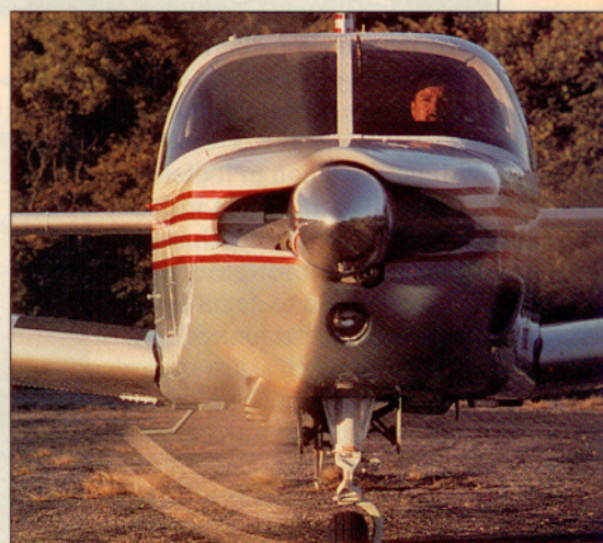
Round cooling inlets and a recessed NACA scoop decrease drag on the II HP compared to the 1988 PA-32 (below).
