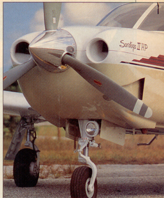
Round cooling inlets and a recessed NACA scoop decrease drag on the II HP compared to the 1988 PA-32 (below).
